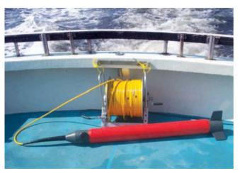
Since SeaSPY's Overhauser technology does not display heading error, no matter how the sensor is oriented in the Earth's magnetic field, successive survey lines taken in opposite directions will match up perfectly.
