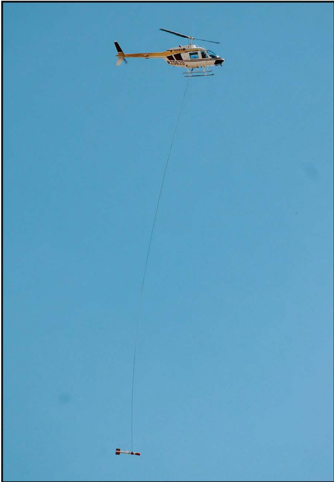
EDCON-PRJ Heli-mag System with Jet Ranger 206B Helicopter
