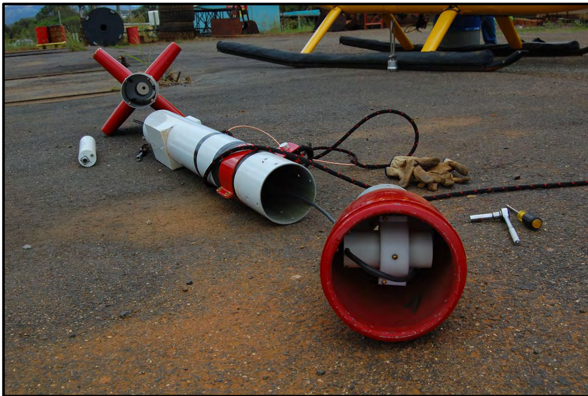
Magnetometer Sensor in Nose of Survey Bird
