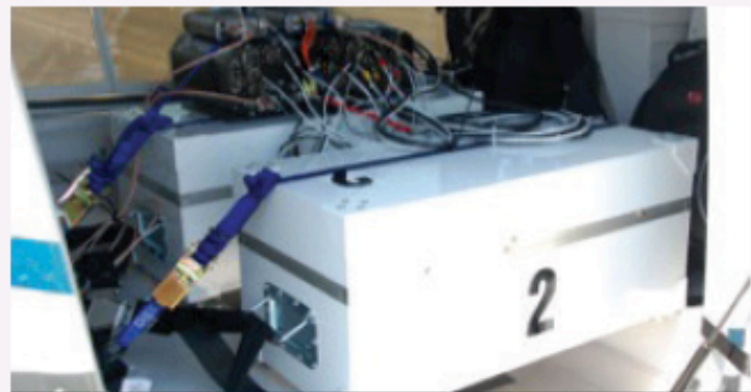
The Advanced Gamma Ray Spectrometer (AGRS System)
