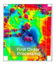
To better image these pipelines and resolve sharper images of the surrounding anomalies, we applied our advanced processing techniques to enhance features that exhibit discrete magnetic signatures. The advanced processing we utilize for these surveys involves a large number of iterative steps, each designed to amplify the discrete signatures of wells and pipelines while maintaining the integrity of the original data.
